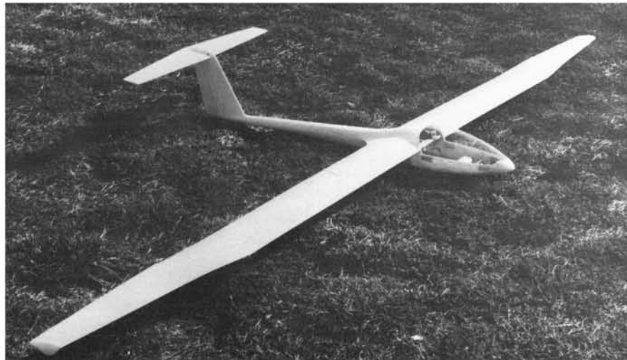
Below: Chet Atkin's scale Caproni spans 11 ft., weighs 8.5 lbs., fiberglass fuselage. Scratch-built, it's Chet's threat to '76 competition.
